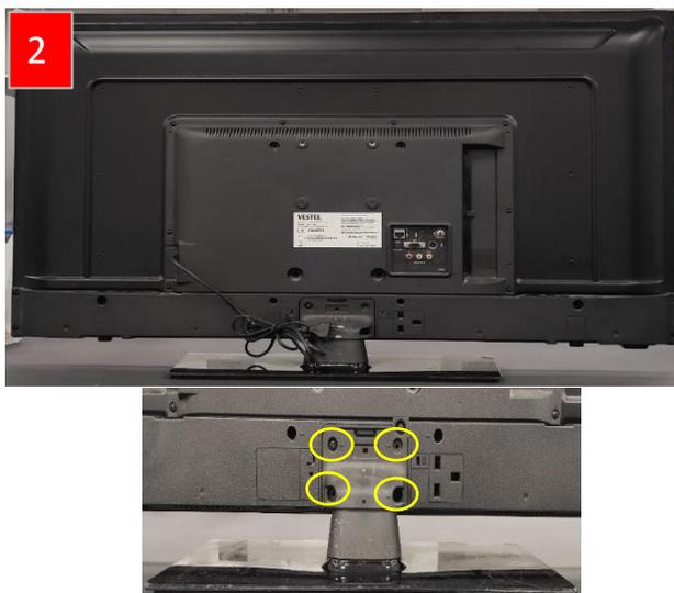
2. Middle stands are disassembled by removing four screws attaching it to TV unit as shown in figure 2
