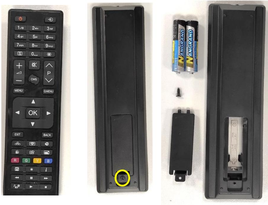
Screw is removed; then backcover and batteries can be taken out.
