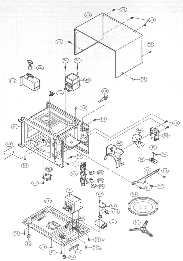
NOTE: In the event of removing the turntable motor cover this part should be refitted using screw connection: LX-CZA030WRE0 (7-11)
