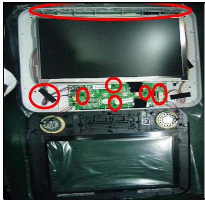
Remove the 4pcs screws and connector on the TFT and IR board.
