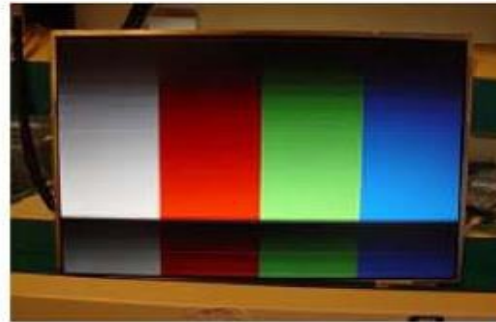
Horizontal Block Gate TAB IC Defect
