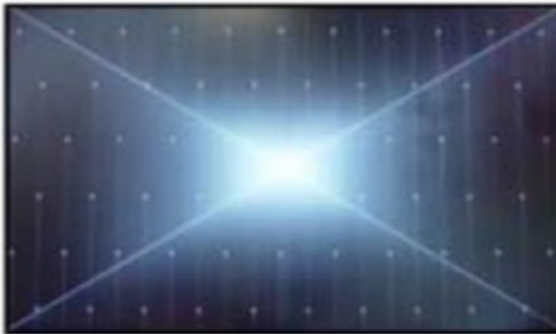
Solder defect, Short/Crack
