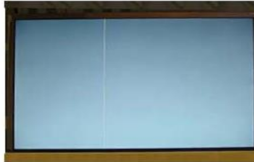
Vertical Line Source TAB IC Defect
