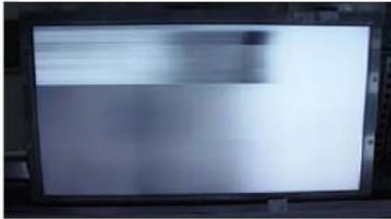
Horizontal Block Gate TAB IC Defect
