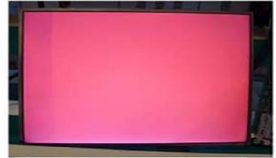
Vertical Block Source TAB IC Defect
