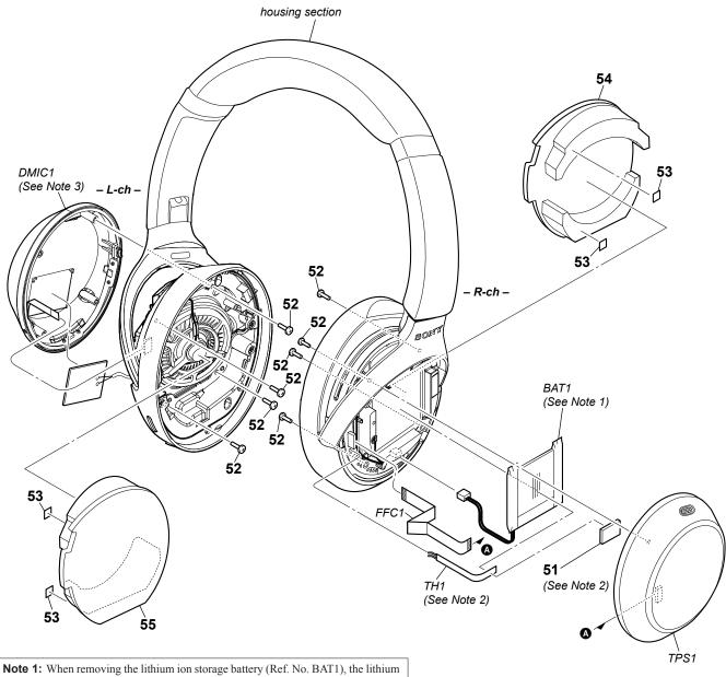
Note 1: When removing the lithium ion storage battery (Ref. No. BAT1), the lithium ion storage battery cannot be reused. Be sure to replace it with a new part. When replacing the lithium ion storage battery, refer to "CHECKING THE NEW LITHIUM ION STORAGE BATTERY FOR BEFORE USE AND NOTES ON HANDLING" on page 4.
