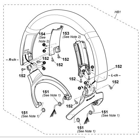
**Note 1:** Lubricant (SANKOL) is applied to the sub cushion AORI assy (Ref. No. 151). Be careful when handling the parts.
