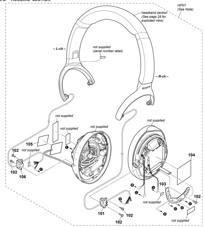
Ref. No. HPN1: Includes the Headband assy, Driver, Electret cap microphone, FFC, Wire, L MAIN board, L NFC board, L JACK board, L KEY flexible board, SUB board and R USB board.
