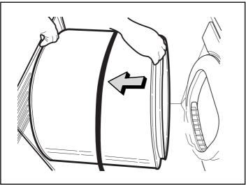
2. Disassemble Drum
