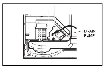
3. Disassemble Drain Pump by unscrewing 2 screws.
