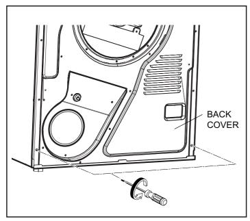
1. Disassemble Back cover from the Base by unscrewing 2 screws.
