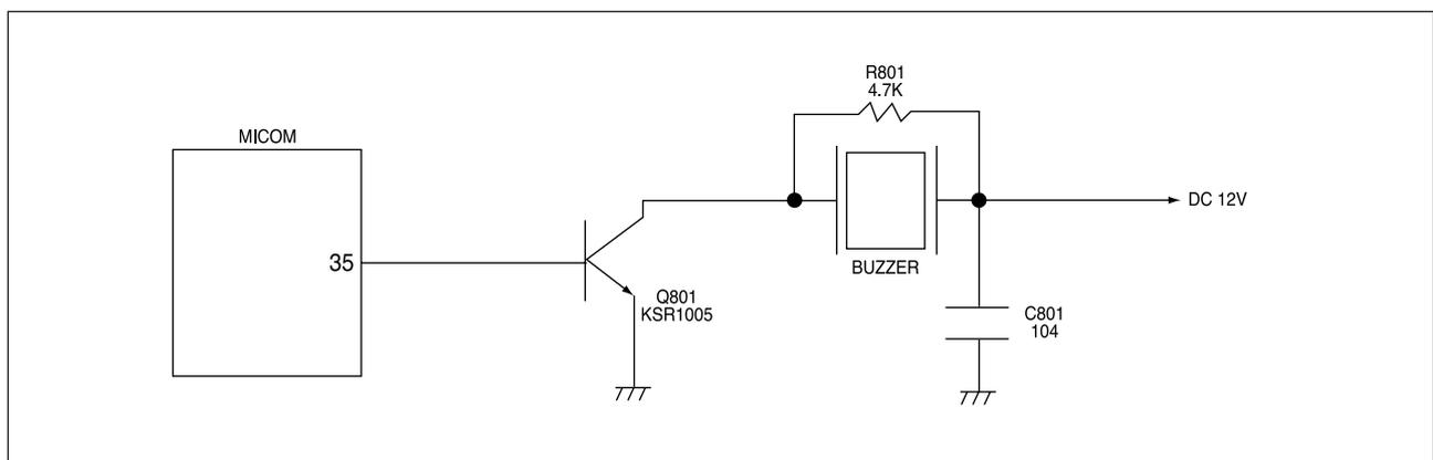
◆ TRANSISTOR begins to operate by CLOCK which was generated at MICOM and BUZZER sound is generated by impression of 12V to the BUZZER.
