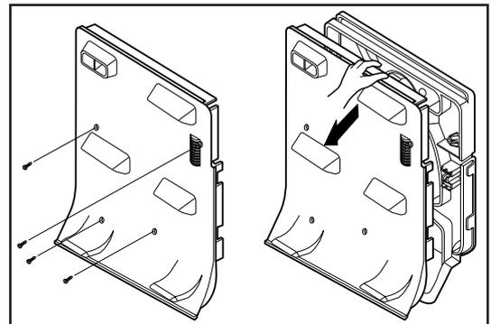
5. Remove 2 screws securing refrigerator duct and pull it out by following the arrow.
