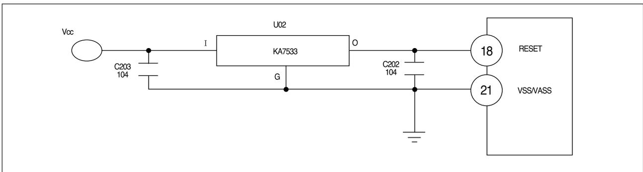
◆ Division of RESET circuit makes it possible that programmed function of system is set to be initial state by initializing various parts such as RAM in MICOM when power is impressed or instantaneous electricity failure is occurred. RESET voltage at the impressed moment of power is maintained as "LOW" state for a few seconds and "High" under normal working condition.
