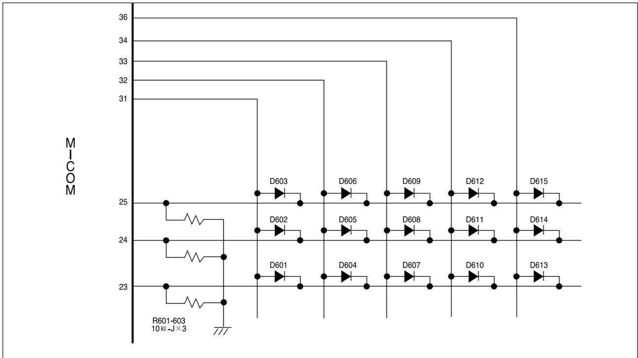
◆ The output such as GRID wave form which is only generated at the initial POWER ON is accepted as input through SWITCHING DIODE and discriminate OPTION by matrix method. #23, #24, and #25 PORT of MICOM PORT generate the same output with GRID wave form only at initial POWER ON.
