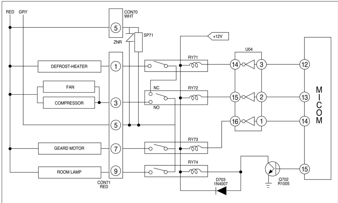
◆ If at MICOM PORT begins to output "High" signal which corresponds to electrical load which we intend to work, DRIVER IC(KA2657) is turned ON and at this moment, corresponding electrical load starts to operate because the DC12V yield the electric current which flows corresponding RELAY COIL and RELAY contacting point is set to be ON so corresponding electrical load begins to operate.
