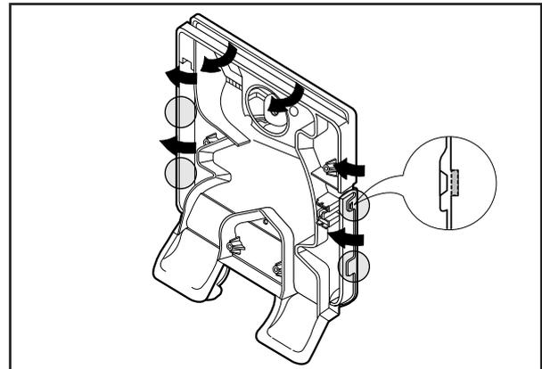
■ Assembly of the cooling cycle unit in the freezer
