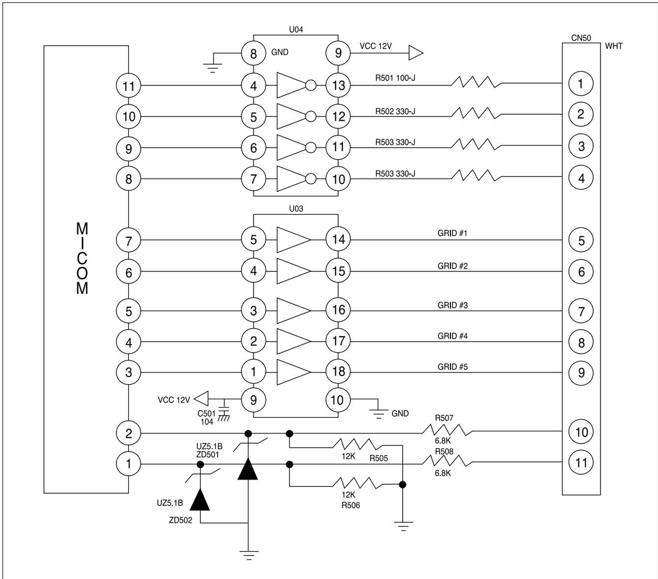
◆ from MICOM #3-#7 GHID signal is generated for 10 sec with the period of 2 sec HIGH signal and for the lighting the corresponding LED, the CONTROL terminal of MICOM PIN #8-#11 output the output signal which is coincident with GRID signal. Meanwhile by pushing the KEY which is connected by respective GRID, corresponding signal is inputted to MICOM.
