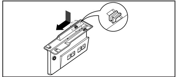
4. Pull forward the insulating material of the cooling cycle unit and remove the wire terminal and insulating material.
