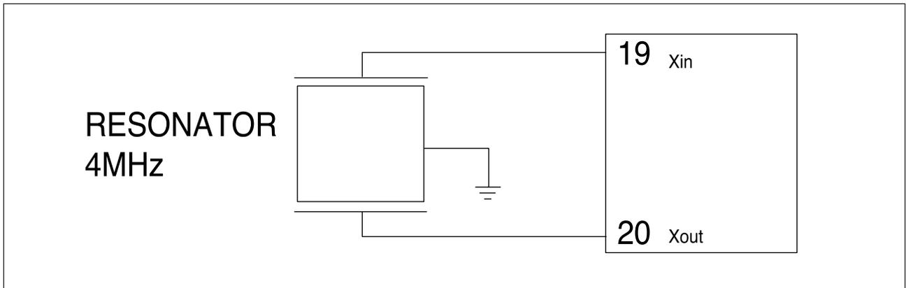
◆ The role of this circuit is generation of synchronous CLOCK for transmission/reception of informations of the logical elements inside MICOM and the basic time for the calculation of time. Rated parts must be used in the division of RESONATOR because the calculation time of MICOM is changed or cannot work if specification is changed.
