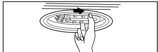
3. After replacing the lamp, assemble the front latch of cover and then connect the back latch and screw on the cover.
