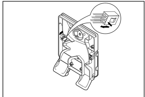
6. Remove 3 screws from the back cover of the cooling cycle unit and remove the latch with (+) driver.
