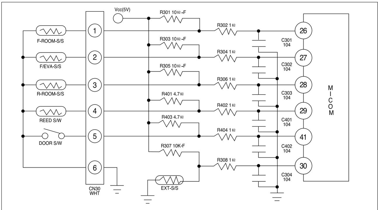
◆ SENSOR and F-rated resistance are connected to the GROUND and DC 5V, respectively. The resistance value which is changed by the temperature is converted to the voltage, and then respective temperature is discriminated by input voltage to A/D PORT of MICOM
