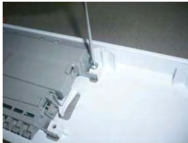
g ) Disassemble by removing the screws retaining the PCB box.
