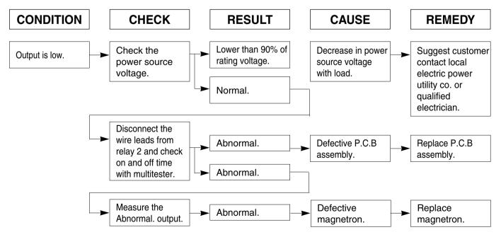
NOTE: Simple test of power output-conducted by heating one liter water for one min. if available.
