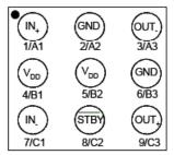
IN+: positive differential input IN-: negative differential input VDD: analog power supply GND: power supply ground STBY: standby pin (active low) OUT+: positive differential output OUT-: negative differential output
