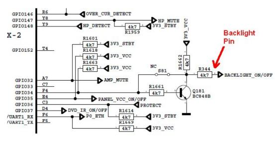
Dimming pin should be high or square wave in open position. If it is low, please check S16 for Mstar side and panel or power cables, connectors.
