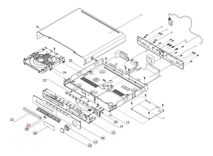
It is general mechanical exploded view for HTS3520/12, detailed information pls refer to the model set. ASSY1 includes components:15.16.19.20.21 ASSY2 includes components:17.18
