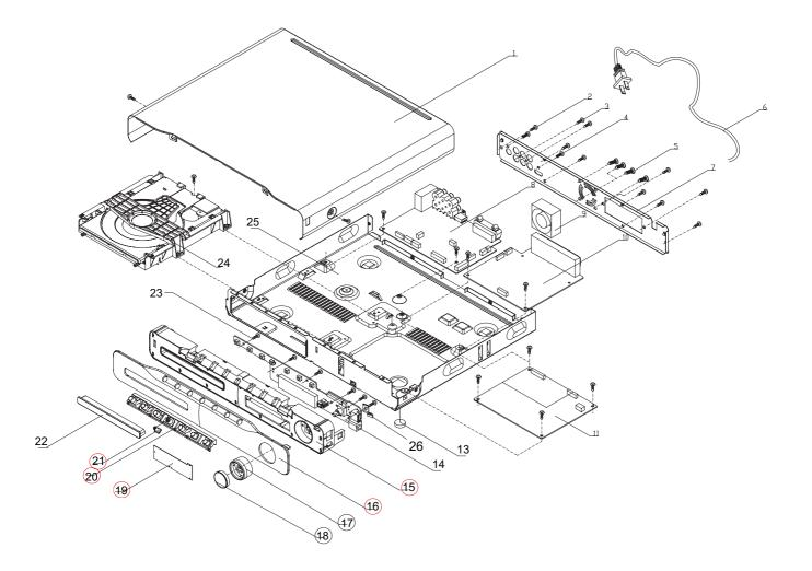
It is general mechanical exploded view for HTS3520/51/X78/94, detailed information pls refer to the model set. ASSY1 includes components:15.16.19.20.21 ASSY2 includes components:17.18
