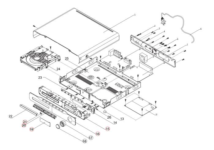
It is general mechanical exploded view for HTS3520/05, detailed information pls refer to the model set. ASSY1 includes components:15.16.19.20.21 ASSY2 includes components:17.18 Exploded view for HTS3520/55/98:
