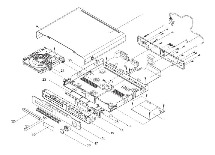
It is general mechanical exploded view for HTS3520/55/98, detailed information pls refer to the model set. ASSY1 includes components:15.16.19.20.21 ASSY2 includes components:17.18
