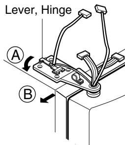
**Note :** • When disconnecting refrigerator door, turn hinge lever counterclockwise.
