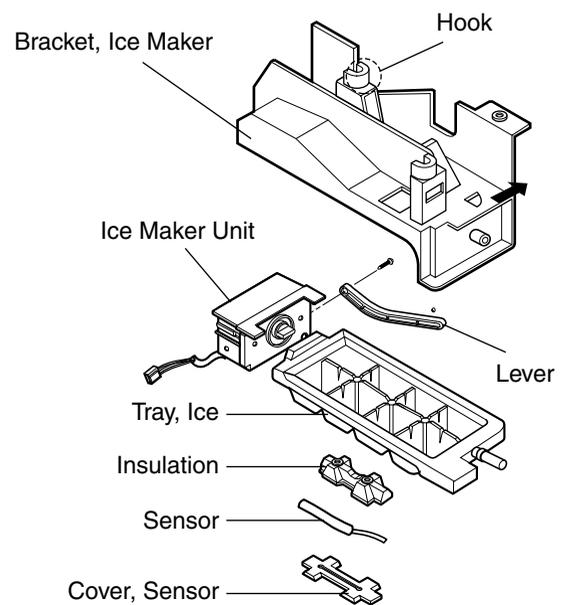
**Note :** When the ice tray is not horizontal after assembly, assembly must be wrong. Check and assemble again.
