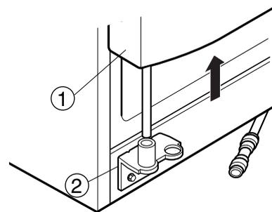
**Note :** • Lift up a freezer door until a water supply tube is fully taken out.
