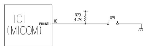
The above circuits are used for designating separation by model as option and notifying it to MICOM. Designation of option by model and the application standards are as follows:
