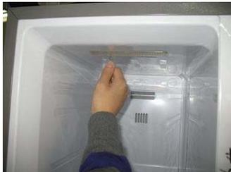
Separate back side of a LED cover using (-) driver.
