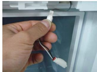
Grip lead switch end connector by hand.
