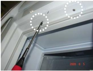
Open home bar door and loosen latch cover fixing screw at upper part of a home bar.
