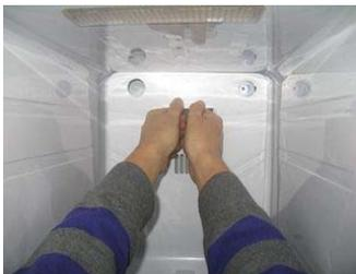
Grip cooling air discharge port of a cooler fan cover and pull it forward direction to separate it from lock.
