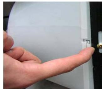
Push and pull forward lock of a bell mouth and separate bell mouth ass'y. (Be careful blade of a fan not to be deformed during disassemble)
