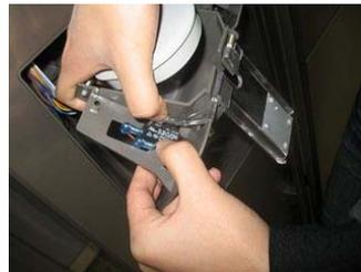
Open up fixing hook and pull out micro switch which is assembled at rear side of a dispenser guide.
