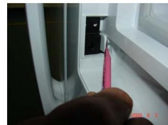
Separate damper support using blade as left side figure.
