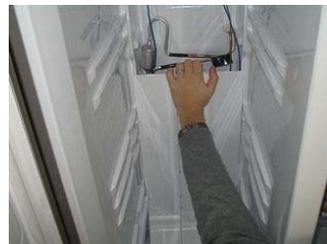
Grip upper part of a cooler front cover by hand and pull it forward direction to separate it.
