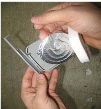
Flap heater can be separated when pull out cushion seal material inside of a flap lever.
