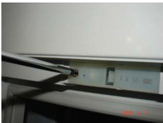
Remove latch fixing screw.
