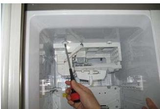
Loosen 2 fixing screws at roof of a freezer and pull a ice maker toward forward direction to separate it.
