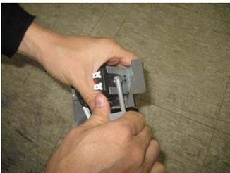
Grip solenoid valve of a flap lever which is assembled at dispenser guide by hand and pull it upper side.
