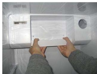
Grip lower side of a damper cover and pull it forward to separate it.
