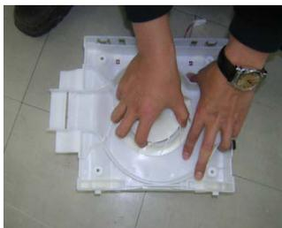
Pull out fan assembled at inner side of a fixture fan motor to vertical direction. [ Fan separation]
