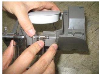
Separate a dispenser lever by pulling it along shaft direction where dispenser lever spring is assembled.
