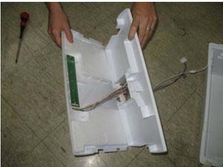
Separate PCB box from changing room cover and disconnect harness between main PCB and front PCB.
