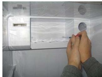
Loosen 2 screws inside of a damper cover.
