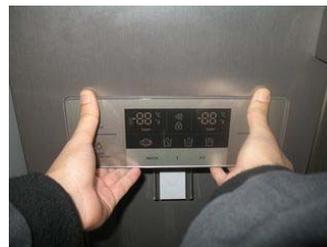
Grip bottom side of a FBC with two hands and lift and pull it forward side to separate FBC.
