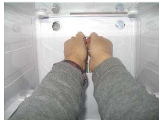
Grip cooling air discharge port at fan cover of a cooler by hand and separate it from lock.
