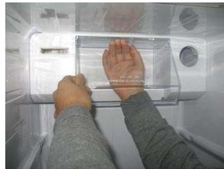
Open window of a damper cover and bend it lightly at center part to separate window.
