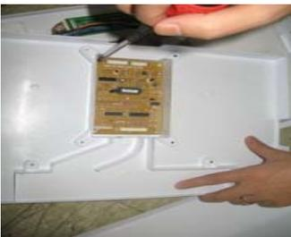
Separate PCB by loosening fixing screw of a Main PCB & Front PCB.
