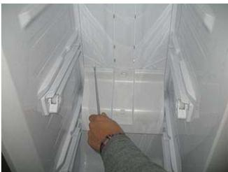
Separate hooks using (-) driver by twisting it which is assembled at return cover and front cover.
