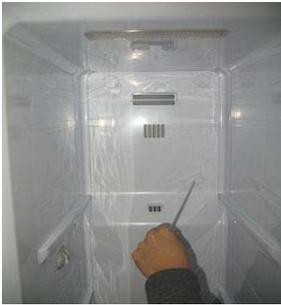
Remove screw cap of a cooler fan located at rear upper side of a freezer.
