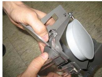
Separate a dispenser lever shaft by lifting one side of a dispenser lever up side along sloped shape home.
