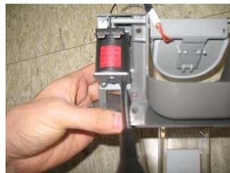
Loosen solenoid valve fixing screws.
