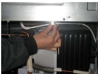
Separate C-fan motor housing at upper right part of a machine room.
