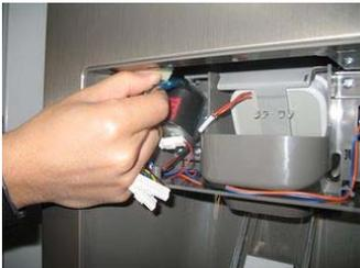
Pull out harness connected to Solenoid Valve. Be careful harness does not be damaged.
