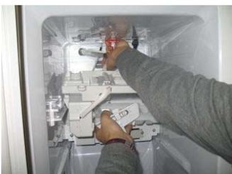
Disconnect harness connected to a ice maker and separate ice maker from a freezer.
