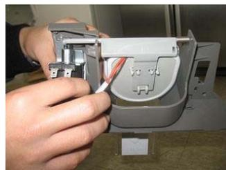
Separate solenoid valve by pulling it down wards and pull out solenoid pin by rotating flap lever.
