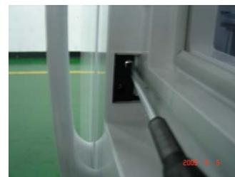
Separate damper fixing screw.
