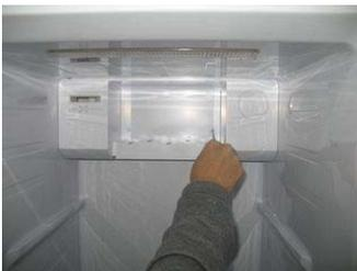
Loosen 2 screws at inside of a damper cover.
