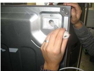
Push back a water supply pipe located at back side of a freezer and go to back side of a refrigerator and pull out a water supply pipe.
