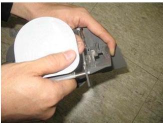
Separate a flap lever completely by pulling it along shaft direction where flap lever spring is assembled.
