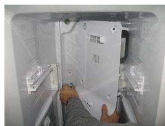
Lift up right side of a cooler fan cover to forward direction and tilt it to disconnect and pull out fan harness located at left side of a cooler fan cover.
