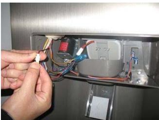
Separate a housing of a dispenser flap heater.
