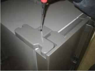
Loosen 2 hinge cover fixing screws.
