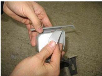
Separate a silicon rubber at flap lever.
