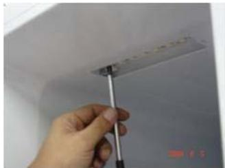
Separate LED cover and loosen 2 fixing screws for LED plate.
