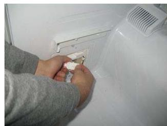
Disconnect harness connected with a damper and pull out a damper.
