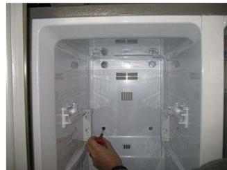
Loosen fixing screw for a fan cover of a cooler.
