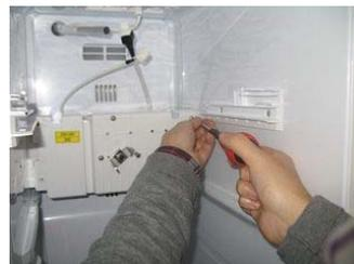
Loosen 4 fixing screws for a Geared-Motor box.
