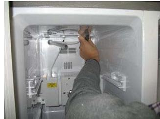
Disconnect 2 kinds of harness which is connected with a Geared-Motor box at upper part of a freezer.
