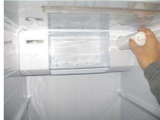
Remove interior filter at right side of a damper cover.
