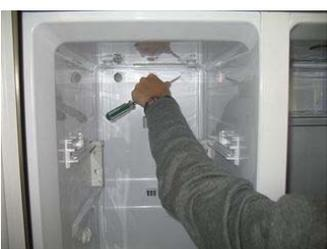
Remove screw cap of a fan cover located at upper rear side of a freezer.
