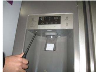
Loosen screws at bottom side of a FBC of a freezer dispenser.
