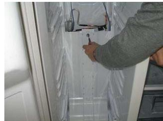
Loosen a fixing screw at cooler front cover.
