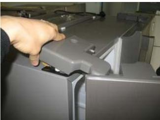
Open door and lift up rear side of a hinge cover and disassemble it.
