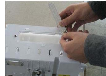
Disconnect harness from LED plate and change LED.
