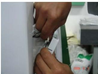
Disconnect 2 harnesses connected with FBC and separate FBC completely.
