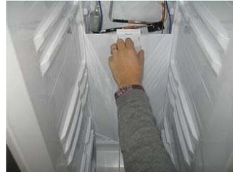
Grip upper part of a duct cover which is assembled at center of a cooler front cover and pull it out to forward direction to separate.
