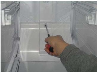
Loosen a screw at center of a return cover.
