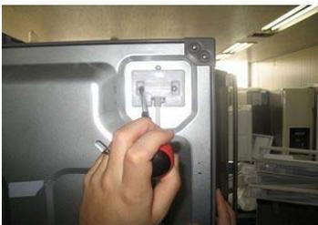
Separate cover & water supply port (silicon rubber) by loosening screw at cover of a water supply pipe at back side of a refrigerator.
