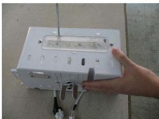
Separate back side of a LED cover located at bottom of Geared-Motor Box using (-) driver.
