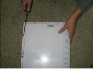
Lift up a hook at back side of a changing room a little bit using (1) driver and pull out a changing room cover to separate it from a changing room.
