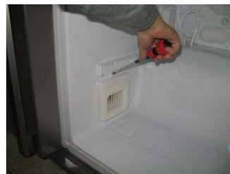
Loosen a screw of a damper cover assembled at left side of a refrigerator.
