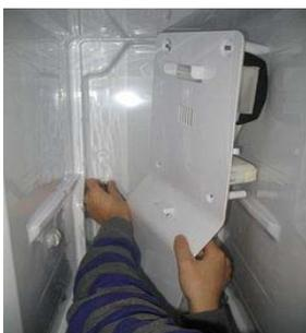
Lift up right side of a cooler fan cover to forward direction and tilt it to disconnect and pull out fan harness located at left side of a cooler fan cover.
