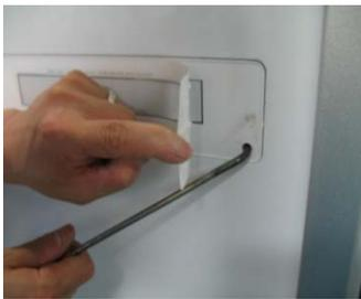
Separate a FBC from a refrigerator at a hole on the film removed area.
