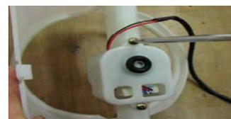
Loosen screws of a motor cover and separate cover and pull out C-fan motor.
