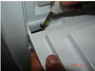
Insert (-) driver at shaft head and grip and pull home bar door with the other hand.
