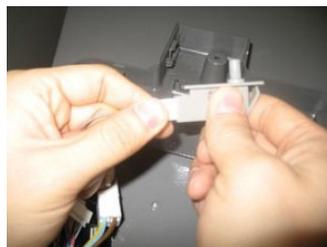
Separate the Harness connected to the Door Switch.
