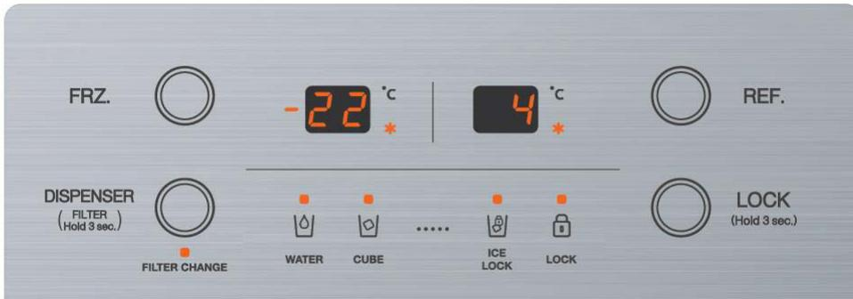
Start: Press “Freezer” Button at “Locked” state and touch “Lock Setup” Button 5 times.
