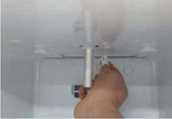
Separate the water-supplying Pipe heater connection socket.
