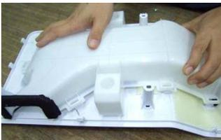
Release the temporary hook of the Louver F A to separate the Louver F C.
