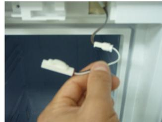
Make the Home-bar Door Switch protrude out of the fixing hole.
