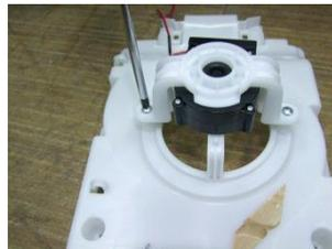
Unwind the fixing bolts (2ea).
