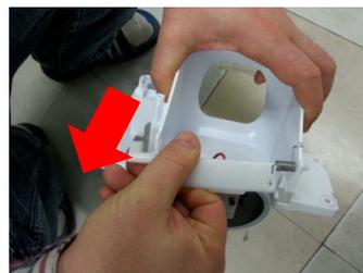
Separate the Flap Lever Rotation Axis from the Ice Shutter and pull it to the direction of the arrow to separate it from the I/SHUT BOX.
