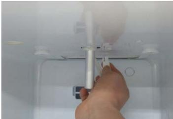
Separate the water-supplying pipe heater connection socket.
