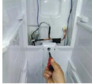
Unwind the bolt (1ea) fixing the Louver F B to the Freezer.
