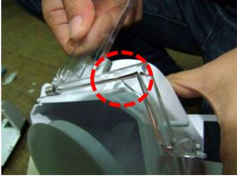
Pull the Dispenser Lever toward the Flap Lever, and take the Display out of the I/SHUT BOX.
