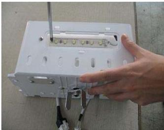
After separating the LED cover, unwind the fixing bolts (2ea) on the LED board.
