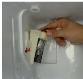
Separate the Damper from the Freezer.
