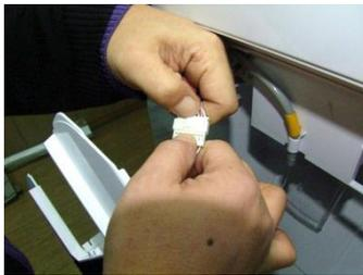
Separate the socket connected to the FCB.
