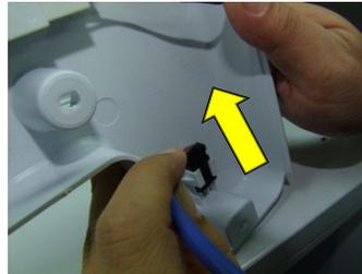
Take out the Humidity Sensor to the direction of the arrow, lifting it up.
