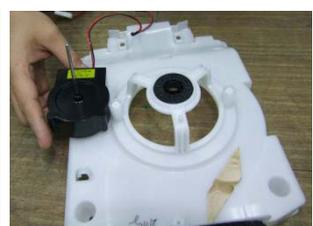
Separate the Fan Motor from the Motor fixing hole.
