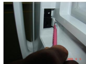
Separate the Damper Supporter, using a knife blade, as in the picture.
