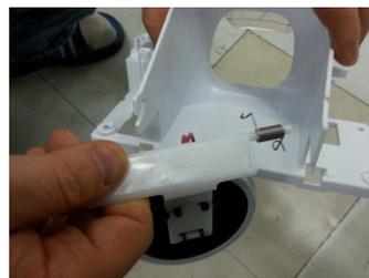
Take the Flap Lever Rotation Axis (Spring interposition) out of the I/SHUT BOX.
