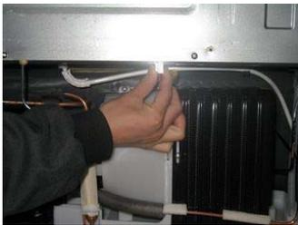
Separate the C-Fan Motor connection socket at the top to the right side of the machine room.
