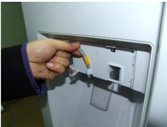
Pull out the water hose from the fixture of the I/SHUT BOX.
