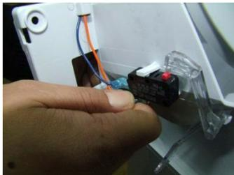
Separate the sockets (2ea) connected to the microswitch attached to the I/SHUT BOX, and pull the harness off the harness holder.
