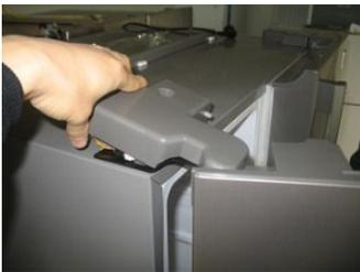
Open the Door and disassemble the Hinge Cover, lifting it from the back of it.
