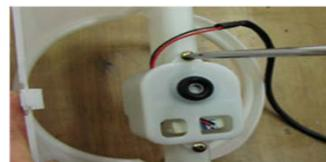
Unwind the bolts of the Motor Cover, and separate the Cover before pulling out the C-Fan Motor.
