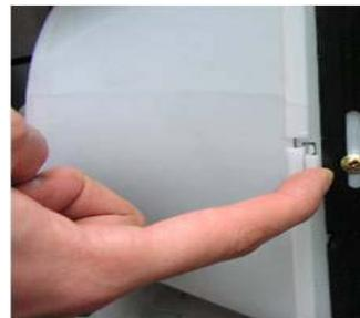
Draw the the Bellmouth toward the front, pressing Lock of the Bellmouth, to separate the Bellmouth Ass'y. (In separating it, take care not to have the fan blades deformed.)
