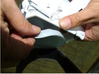
Separate the silicon rubber of the Flap Lever.
