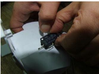
Pull off the Microswitch by opening the fixing hook of the I/SHUT BOX.
