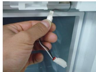
Hold the Lead Switch Socket with a hand.
