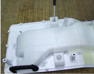
Unwind the Louver F C fixing bolts (3ea).
