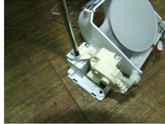
Unwind the fixing bolts (3ea) of the Ice Shutter.
