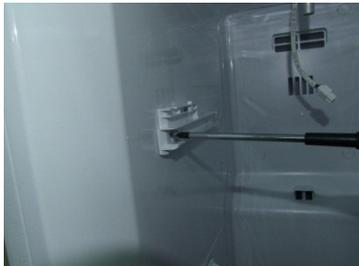
Unwind the fixing bolts (2ea each) of the ice shaver guides fixed to the left and right side of the Freezer and separate them from the Freezer.
