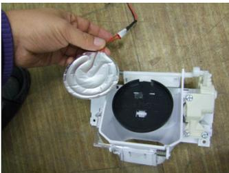
Pull the Heater off Flap Lever.
