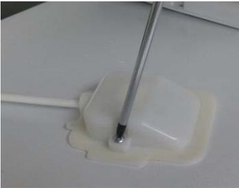
Unwind the bolt of water-supplying pipe cover at the top of the refrigerator and separate the cover from the water-supplying outlet (silicon rubber).
