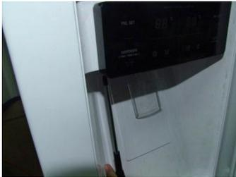
Unwind the bolts at the bottom of the FCB of the Freezer Dispenser.
