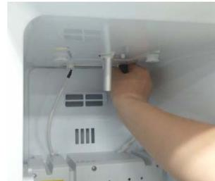
Separate the two connection sockets connected to the Geared-Motor Box at the top of the Freezer.
