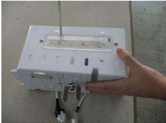
Insert a (-)driver into the rear part of the LED cover at the bottom of the Geared-Motor Box and pull it toward the front to separate the LED cover.
