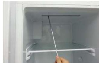
Insert a (-)driver into the rear part of the LED cover and pull it toward the front to separate the LED cover.
