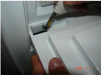
Insert the (-)Driver to the Shaft Head and pull it, holding the Home-bar Door with one hand.
