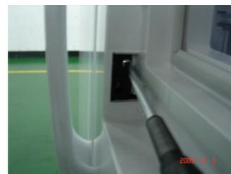
Separate the Damper-fixing bolts.
