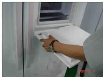
Separate the Home-bar Door from the refrigerator by orderly twisting it from its left side.
