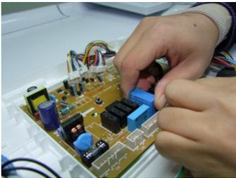
Pull the connection sockets off the Main PCB.
