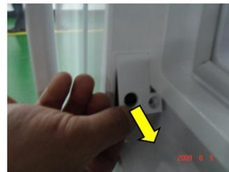
After unwinding the bolt, pull the Cover Damper to the direction of the arrow, using a tool to separate it.
