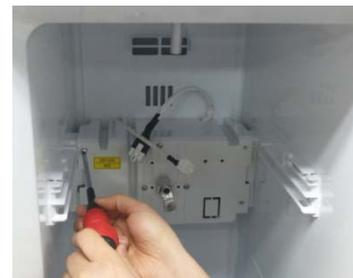
Unwind the fixing bolts (4ea) of the Geared-Motor Box and separate it from the Freezer.
