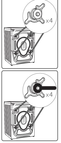
For this reason, transportation safety screws shall be loosened by being rotated in counter-clockwise using an appropriate wrench.
