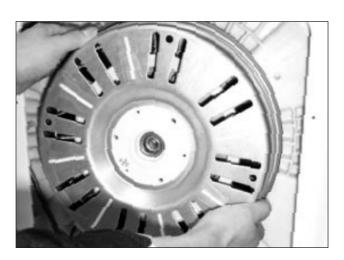
4) Separate the STATOR from the TUB.
