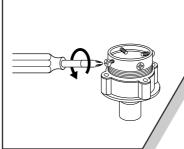
(3) Fit the water tap adapter into the water tap and tighten the four screws evenly while pushing up the adapter so that the
