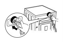
• Check the packing in the inlet.
