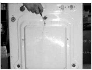
2) Remove the connectors of the HEATER.
