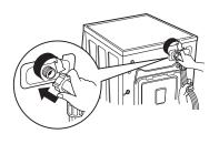
· Check the packing in the inlet.
