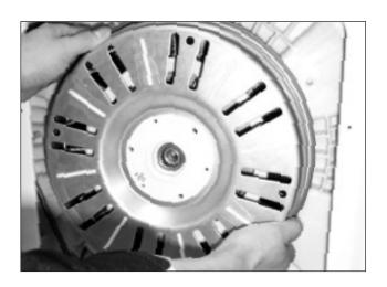
4) Separate the STATOR from the TUB.
