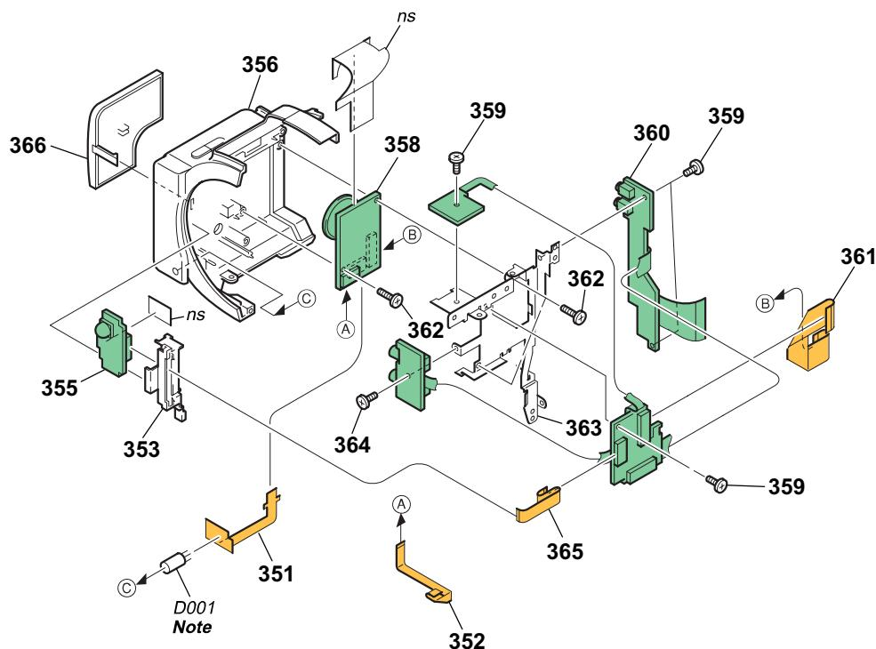
*Note: Adjustment is needed when laser unit (D001) is replaced.*
