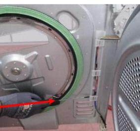
5. Remove the cable group by opening the cable holder plastic canal.
