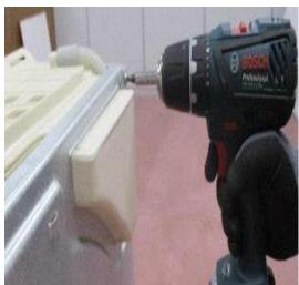
1. Remove the screws on rear panel.
