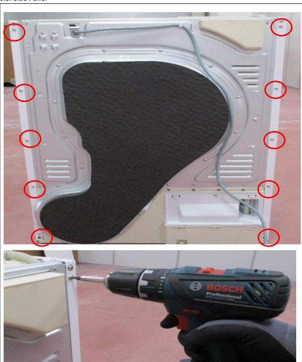
1. To remove the side panels, first remove the 5 screws for each panel at the back.
