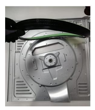
1. For disassembling the rear Isolation group on rear panel, screws are shown in the photo should be removed.
