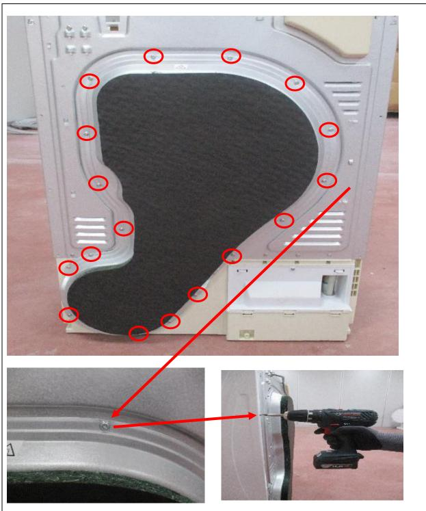
1. Remove all screws on the rear cover shown in the picture.
