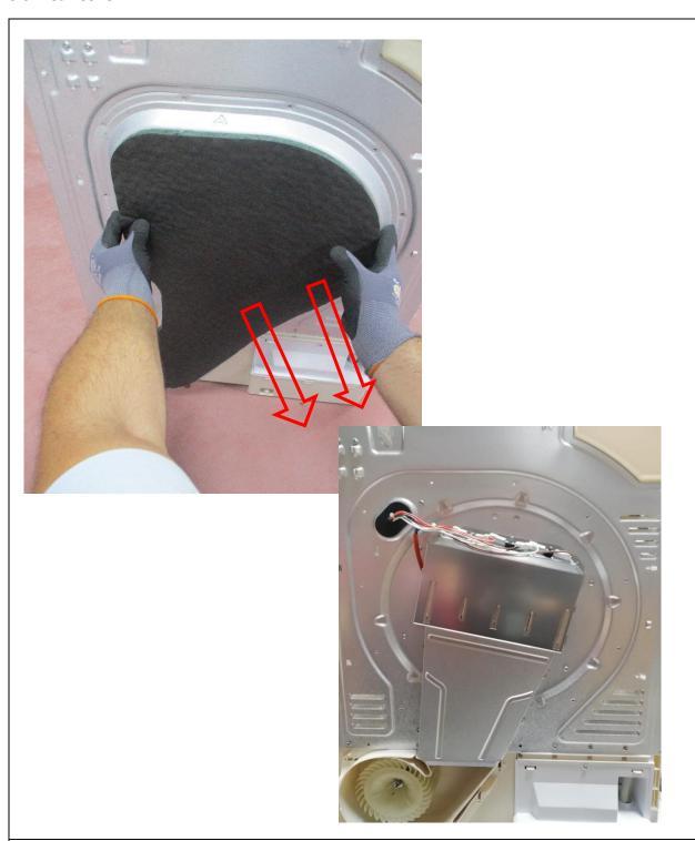
2. Disassemble the rear cover after the screws have been removed.
