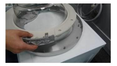
6. Remove six screws that fix the door hinge as it is shown in the picture.
