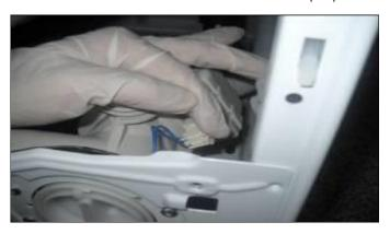
Remove four screws fixing the pump motor.
