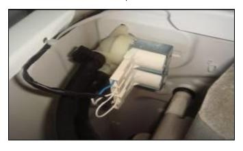
3. Turn the feed valve counter clockwise slightly to remove.
