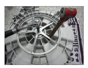
2. Remove the driven pulley it is shown the picture.
