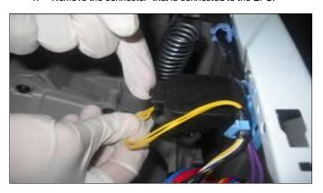
2. Pull the EPS upward to remove as it is shown in the picture.
