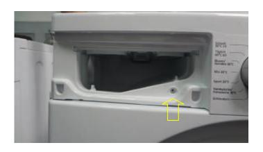
2. Remove three screws fixing the control panel.
