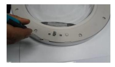
5. Remove the door inside plastic as it is shown in the picture.
