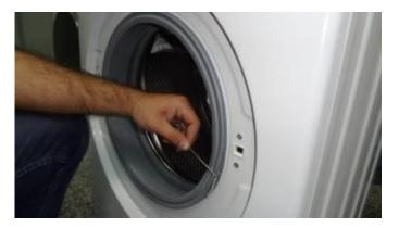
2. Remove the tub bellows seal-body fixing spring.
