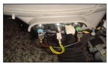
Remove one nut fixing the heater slightly (box wrench size 8 mm)
