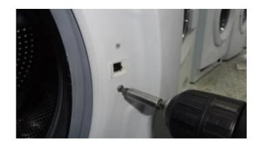
5. Remove two screws fixing the body group at the front as it is shown in the picture.
