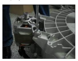
2. Pull the motor up for disassembly.
