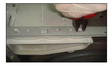
Remove the tub seal clamp by using the pliers, which is attached to the detergent drawer housing.
