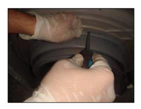
2. Hold the tub bellows seal and gasket-body fixing spring together, and pull them up.
