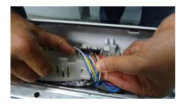
6. Remove electronic card cover as it is shown in the picture by using small screw driver.
