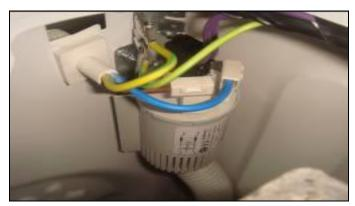
2. Remove two screws fixing the parasite filter.
