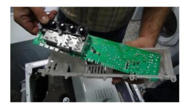
8. Push clips to remove to selection button as it is shown in the Picture.
