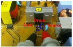
Fig. 7 Q501 Drain-Source measurement
