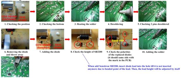
Fig. 5 D210 & D501 Replacement flow
