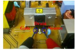
Fig. 8 Q501 Gate-Source measurement
