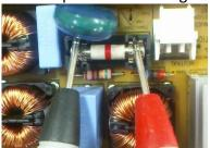
Fig. 9 Fuse F101 measurement
