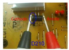
Fig. 10 Diode **D501** & D210 measurement
