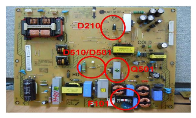
Fig. 1 Location of components D210, D501, Q501, and F101
