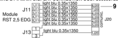
WIRING B = SELECTION CONNECTION COD. C00093723
