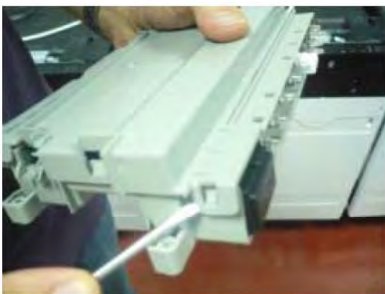
h ) Open the tabs of the PCB box (as shown in the picture) with a flat head screwdriver (take care not to break the plastic part)
