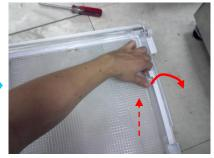
\*When assembly the vegetable tray, insert the boss to the hole like down picture.
