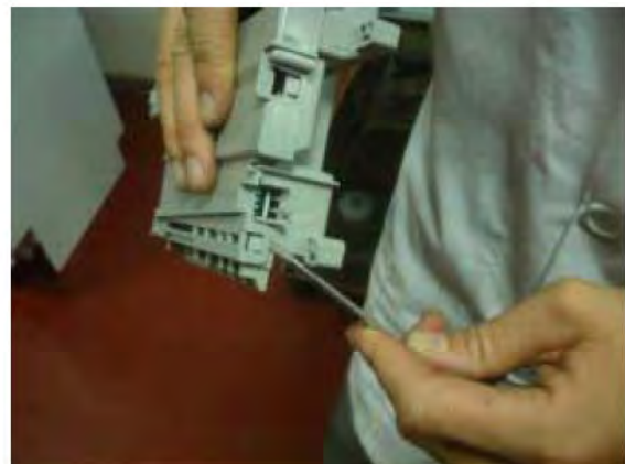
h ) Open the tabs of the PCB box (as shown in the picture) with a flat head screwdriver (take care not to break the plastic part)
