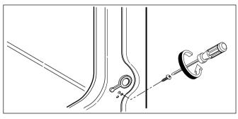
② Unscrew the single screw from the lower-right side of the cabinet.
