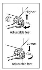
If it is not stable, adjust feet accordingly. After the washer is level, tighten the lock nuts up against of the base of the washer. All lock nuts must be tightened. If it still has severe vibration and noise, regulate a specific spin speed that generates excessive vibration and noise as follows:
