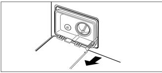
③ Put a flat ( – ) screwdriver or putty knife into the both sides of the filter cover, and pull it out.
