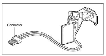
③ Disconnect the connector from PWB Harness.
