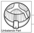
If you do not have the unbalance part, put 4.5 to 6.5 lbs (2 to 3 kg) of clothing. Once loaded, press power, Rinse+Spin and the start/pause button in sequence.
