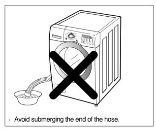
\*\* The end of the drain hose should be placed less than 100 cm from the floor.
