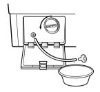
• If SVC is needed during check, remove the remaining water by pulling out the hose cap.
