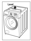
Check the leveling of the washer with a Level and check that the washer is stable.
