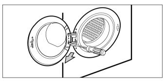
③ Put a flat ( - ) screwdriver into the opening of the hinge, and pull out the hinge cover.
