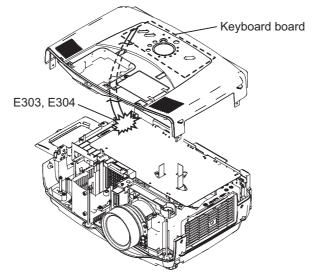
When removing the Drive board, there might be damage to the flexible cables of LCD panels and two board-to-board connectors. Handle them with care when disassembling.
