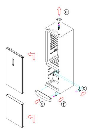
a. Remove 'Top Cover Hinge' and 'Top Hinge'
