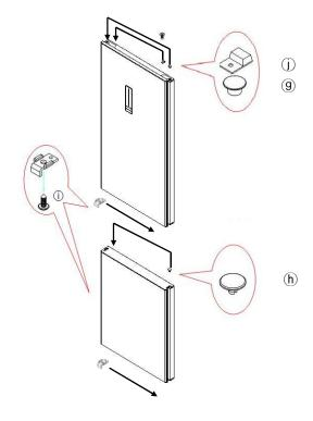
1-3. Reassemble the Freezer and Refrigerator Door
