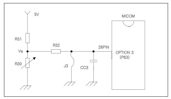
; The input voltage of MICOM and R-Sensor ON/OFF point by changing J3 & R30.
