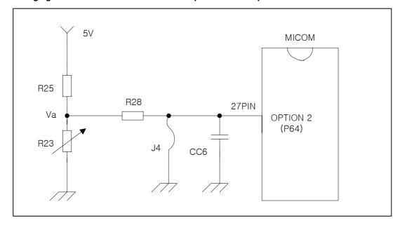
; The input voltage of MICOM and R-Sensor ON/OFF DIFF. by changing J4 & R23.
