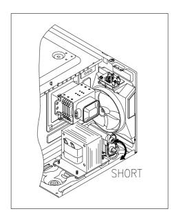
**CAUTION**: Service personnel should remove their watches whenever working close to or replacing the magnetron.
