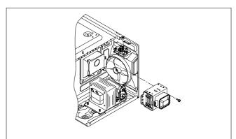
**NOTE**: Never install the magnetron without the metallic gasket plate which is packed with each magnetron to prevent microwave leakage. Whenever repair work is carried out on magnetron, check the microwave leakage. It shall not exceed 4mW/cm² for a fully assembled oven with door normally closed.
