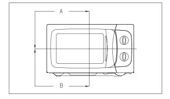
**NOTE**: A small gap may be acceptable if the microwave leakage does not exceed 4mW/cm<sup>2</sup>.
