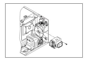
**CAUTION**: Never install the magnetron without the metallic gasket plate which is packed with each magnetron to prevent microwave leakage. Whenever repair work is carried out on magnetron, check the microwave leakage. It shall not exceed 4mW/cm² for a fully assembled oven with door normally closed.
