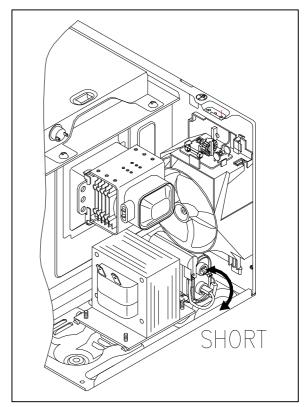
**CAUTION**: Service personnel should remove their watches whenever working close to or replacing the magnetron.
