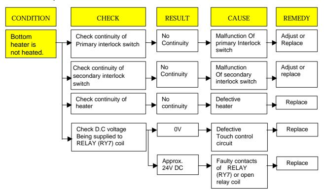
**(TROUBLE 6)** The Following visual conditions indicate a probable defective touch control Circuit or button P.C.B assembly
