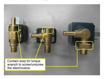
CAUTION #2: Ensure torque wrench jaw does not contact the solenoid body.
