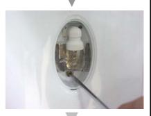
\* Hold top of the MULT DUCT COVER AS and pull forward to remove.
