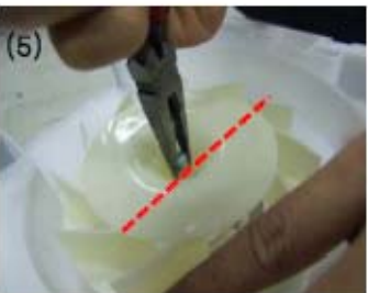
Remove the spring from the Fan.
