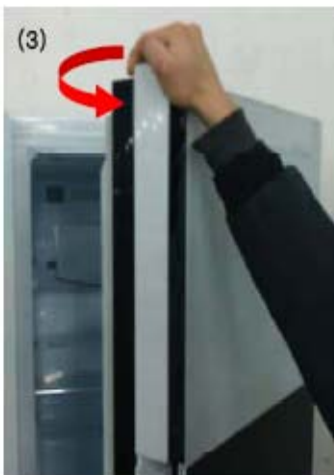
Holding the topside and rotate the FCP Panel CCW.
