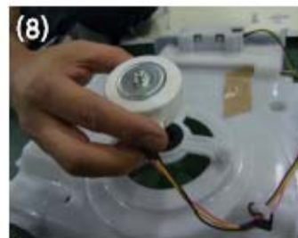
Disassemble the Fan Motor.
