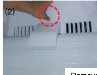
Remove the Air Return Cover pushing the mark point.
