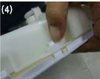
Disassemble with holding the hook.
