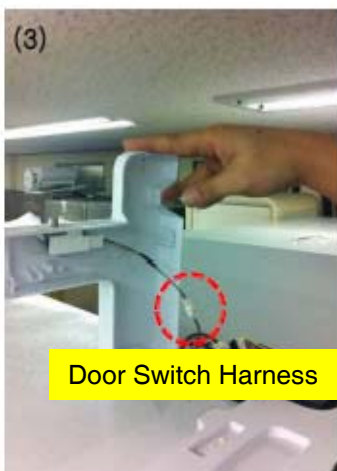
Remove opposite Ref. door switch connector.
