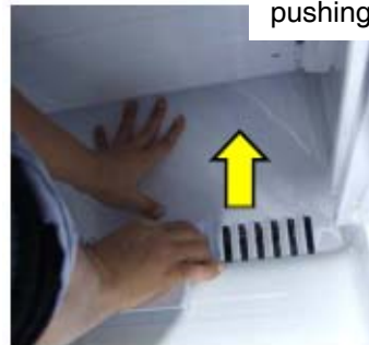
Remove the Air Return Cover pushing the mark point.
