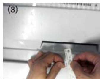
(3) Exchange the LED PCB.
