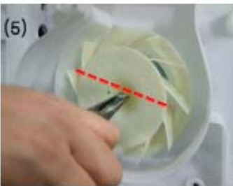
Remove the spring from the Fan.
