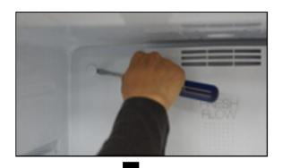
1) Remove screw cap on the Freezer Louver.
