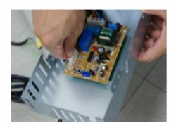
3) Remove the Power Code and harness from the main pcb housing.
