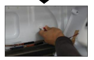
4) Disconnect fan motor lead Wire.
