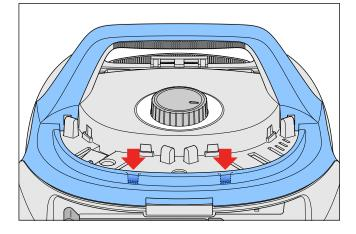
• Then with a small screwdriver lift the Handle cover over the nock on the Top housing (see picture).
