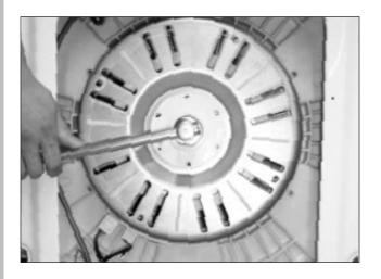
3) Remove six screws using the 10mm hex wrench and connectors from the STATOR.
