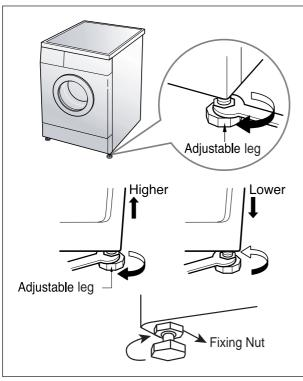
2. If the floor is uneven, adjust the adjustable leg as the following.
