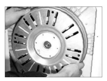
4) Separate the STATOR from the TUB.
