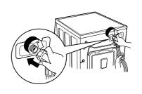
• Check the packing in the inlet.
