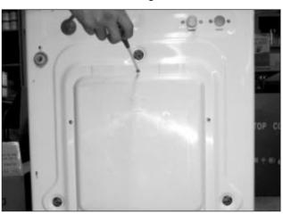
2) Remove the connectors of the HEATER.
