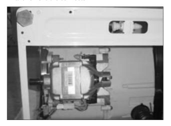
4) Remove the motor from the tub.
