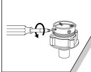
3 Fit the water tap adapter into the water tap and tighten the four screws evenly while pushing up the adapter so that the
