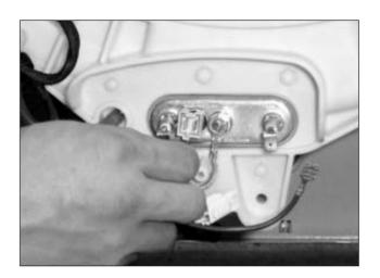
3) Remove the nut using the 10mm hex wrench and remove the earth terminal from the HEATER.
