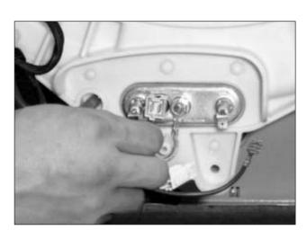
3) Remove the nut using the 10mm hex wrench and remove the earth terminal from the HEATER.
