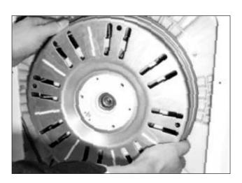
4) Separate the STATOR from the TUB.
