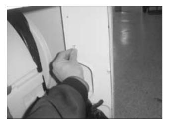
3) Remove the screw, and remove the drain pump from the lower frame.
