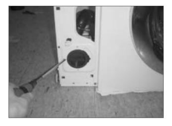
5) Remove the inner drain hose, and remove the drain pump.
