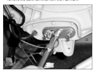
4) Loose the nut of the HEATER and pull out the HEATER.
