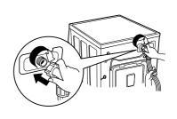
• Check the packing in the inlet.
