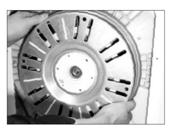
4) Separate the STATOR from the TUB.
