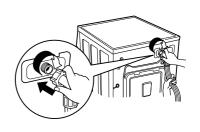
· Check the packing in the inlet.
