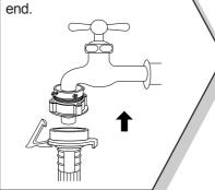
(6) Connect the inlet hose adapter of the hose to the water inlet of the washer by turning it clockwise to be fixed tightly.
