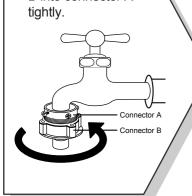
(5) Connect the inlet hose to the water tap adapter by pulling down the collar of the hose
