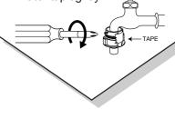
(4) Remove the tape, and screw connector B into connector A
