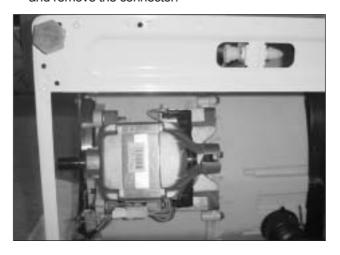
4) Remove the motor from the tub.
