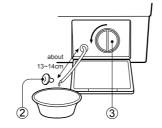
3. Remove any foreign material from the pump filter(③). After cleaning, turn the pump filter clockwise and insert the cap hose(②) to the original place. Close the lower cover.
