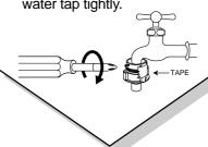
4 Remove the tape, and screw connector B into connect A tightly.
