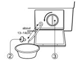
3. Remove any foreign material from the pump filter(3). After cleaning, turn the pump filter clockwise and insert the cap hose(2) to the original place. Close the lower cover.
