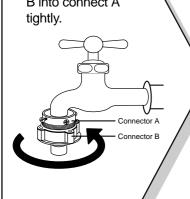
(5) Conect the inlet hose to the water tap adapter by pulling down the collar of the hose end.
