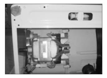
4) Remove the motor from the tub.
