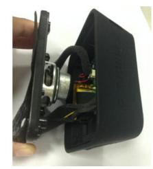
After remove the rubber plugs&screws on the front pannel
