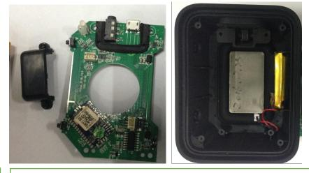
After remove four screws& USB sealed box&unplug the sockets
