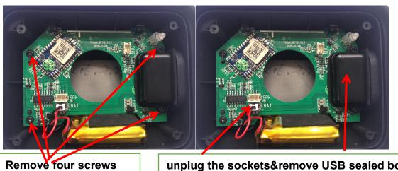
unplug the sockets&remove USB sealed box
