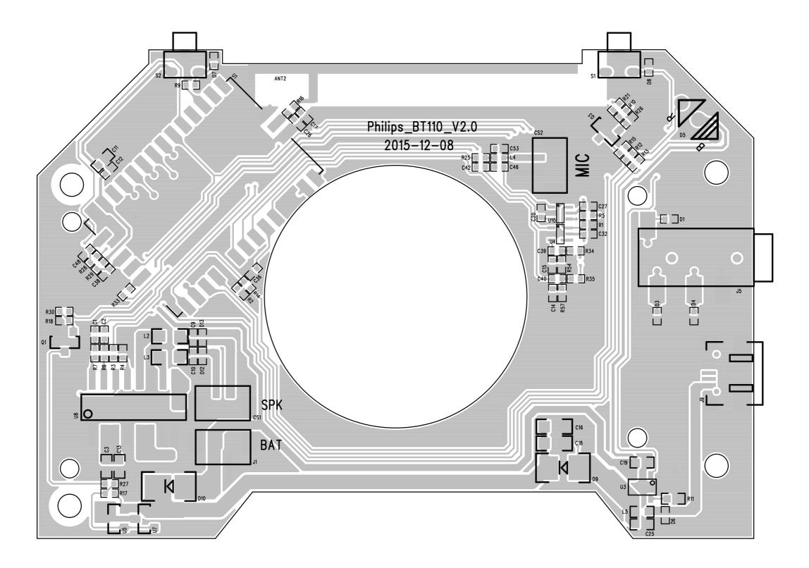
Main board Layout diagram Bottom
