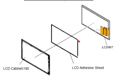
Follow the guidelines below for proper removal / reattachment of "LCD901".
