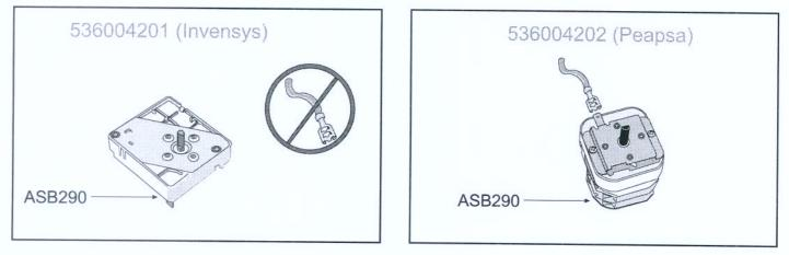
The two types of timer (ASB290) can be fitted to all vented driers without distinction. The only exception being linked to possible fitting problems.
