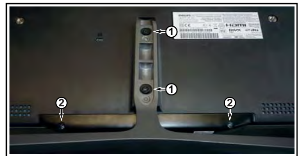
Figure 4-16 Rear cover removal Ambilight models -1-
