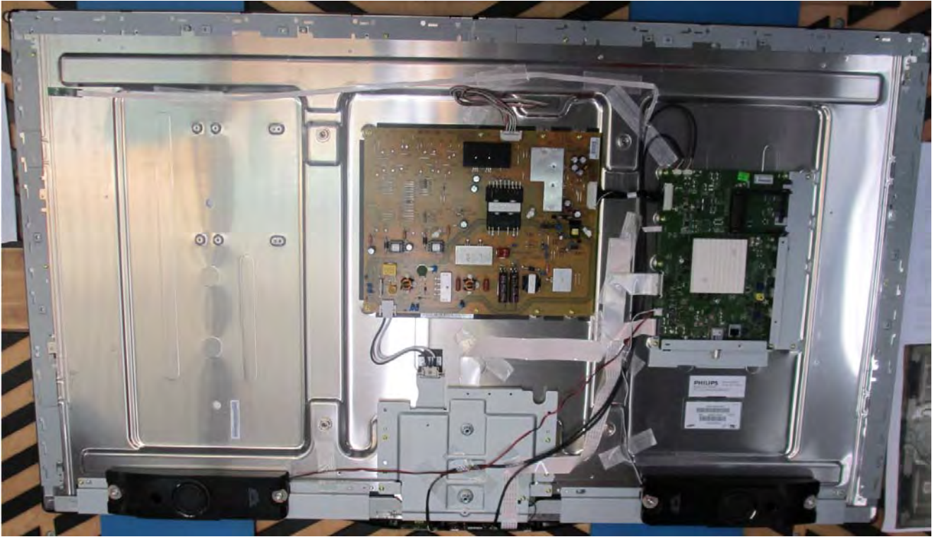
Figure 4-9 Cable dressing 55" 8000 series
