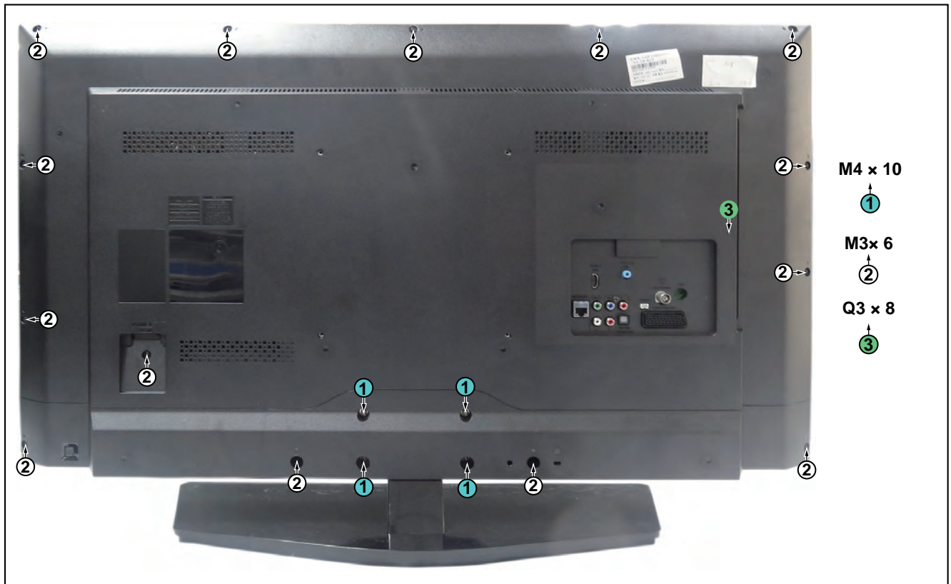
Figure 4-4 Rear cover removal
