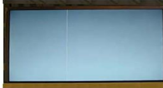
Vertical Line Source TAB IC Defect
