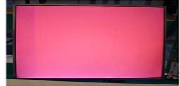
Vertical Block Source TAB IC Defect
